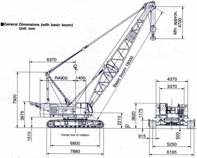
Model KI3C-UV 374PS / 2000 rpm 275 KW / 2000 min
